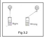
**CAUTION** Do not winch from an acute angle as the wire rope will pile up on one side of the drum causing damage to wire rope and the winch. Fig 3.2 Short pulls from an angle can be used to straighten the vehicle. Long pulls should be done with the wire rope at a 90° angle to the winch/vehicle.
