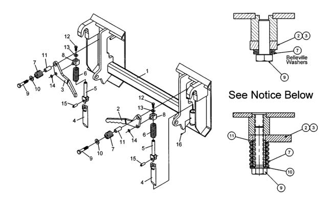
**NOTICE:** Some adapters with the "Universal" Skid Steer connection have 5/8" concave"Belleville" washers to provide tension on the latch handles. Other adapters have a compression spring to provide tension on the latch handles. These parts are **NOT** interchangeable. When ordering replacement parts, check to make sure the correct parts are ordered.
