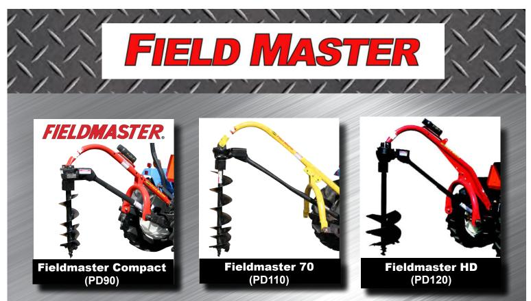
All models include: gearbox equipped with safety shielding for auger and driveline, shielded driveline, yoke, boom, and hardware package. Augers are optional.
