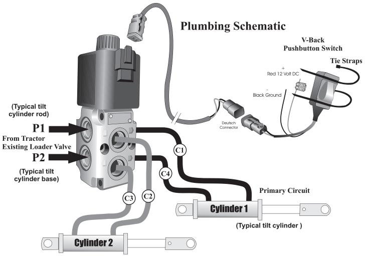
Auxiliary Circuit (Press button) (Typical grapple or 4-in-1 bucket)
