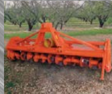
RG Tiller with Adjustable Rear Roller
