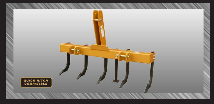
**PA SERIES SCARIFIER ATTACHMENTS** are ideal for breaking up hard ground or renovating pastures. Designed for category 1 tractors up to 50 HP and are available in 5, 6 and 7 shank models. Tool bar widths are 49", 61" and 72". The heavy-duty 4" x 4" x 1/4" tubing is equipped with two position heat-treated forged scarifier shanks with replaceable teeth. Unique shear-bolt shank feature protects your investment. Parking stand included.
