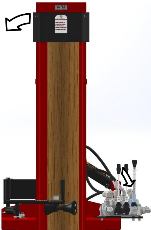
Tilt top of Drive Ram away from operator pull first lever toward operator.
