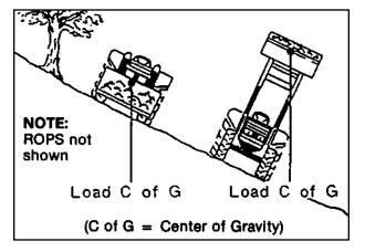
When working on side hills, **DO NOT RAISE LOADER TOO HIGH.** Keep an eye on terrain changes. Keep load low. Make sure all operators have read the Owner's Manual and are familiar with the instructions and the safety rules of operation.
