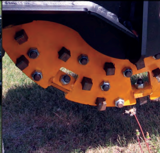
REPLACEABLE TEETH WITH ONE BOLT PER TOOTH
