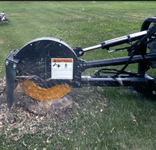
HYDRAULIC CYLINDERS PROVIDE PRECISE HORIZONTAL AND VERTICAL POSITIONING
