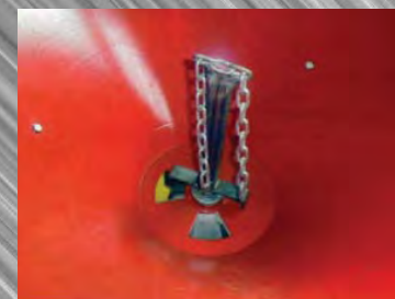
Optional chain agitator to prevent bridging of material
