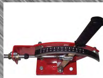
Remote cable control for calibration and shut off
