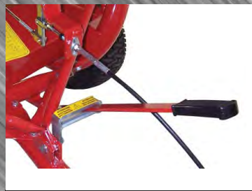
Gearbox lever to disengage drive for transport
