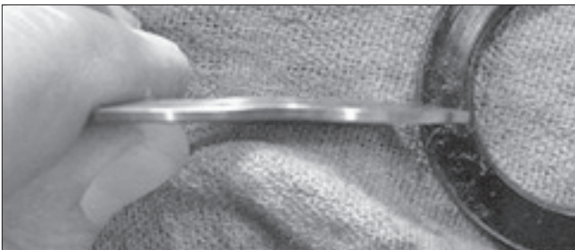
Over-Pressurized Damaged Washer
