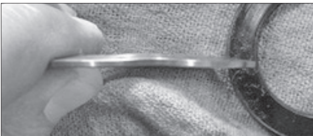
Over-Pressurized Damaged Washer
