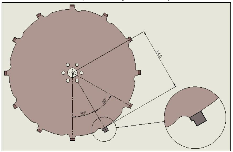
It is recommended to have a chamfer grinded on the rotor edges to have a nice Bevel weld. This will also help balance the weight of the rotor.
