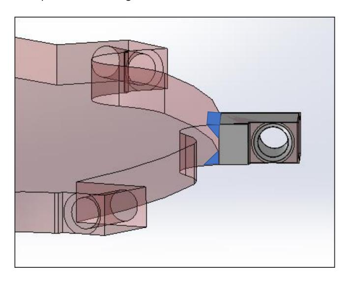
Make sure the face of the of the rotor and tooth holder is inline with each other. Also make suer the new tooth holder does not project out from the overall diameter of rotor 30".
